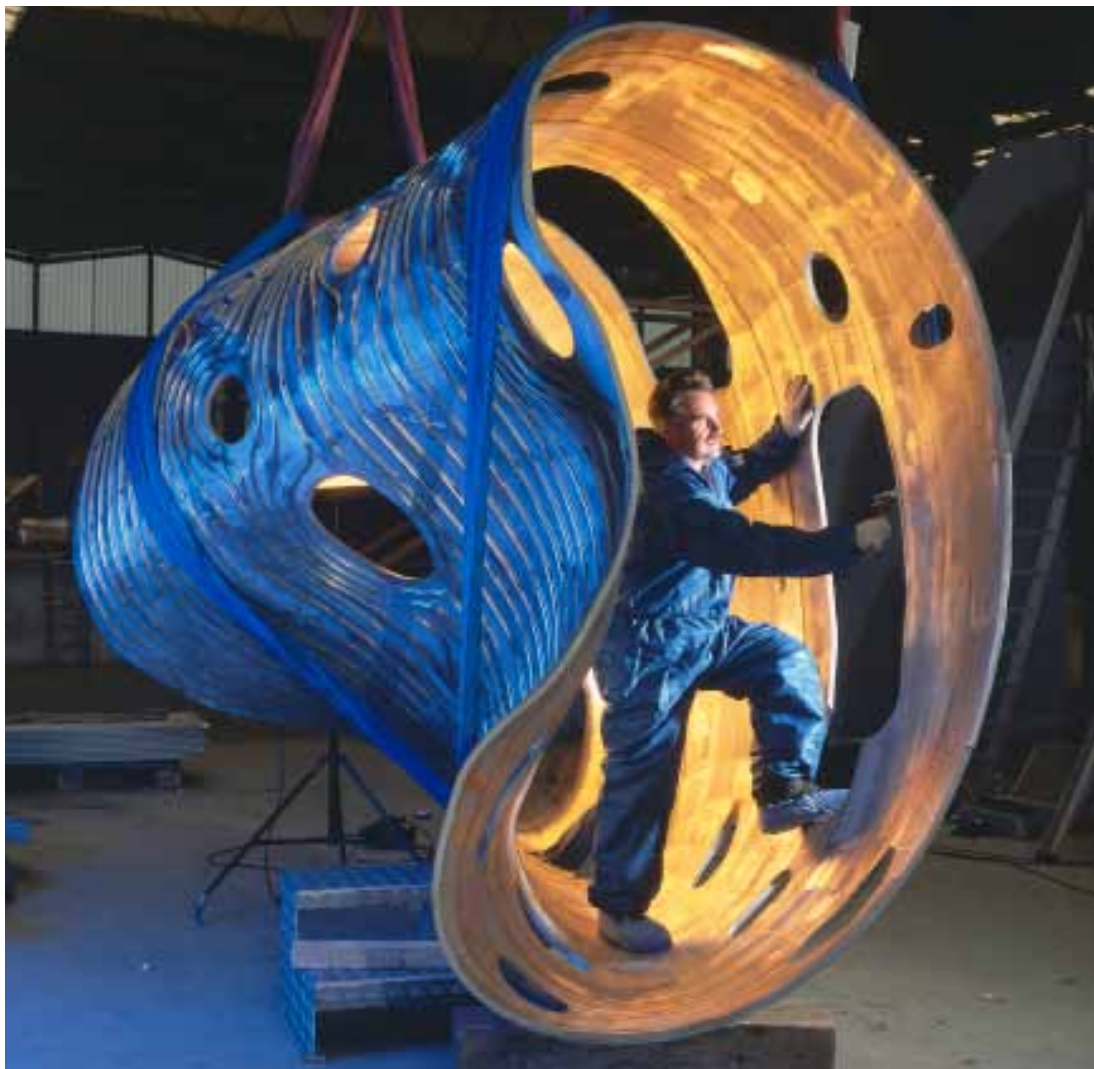
Part of the Wendelstein 7-X plasma container during production
