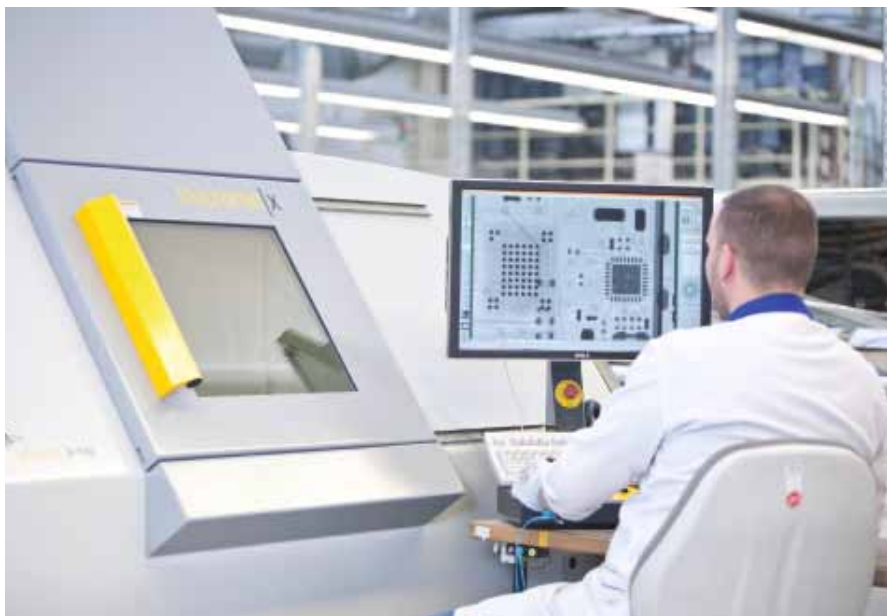
X-ray inspection of an electronic component
